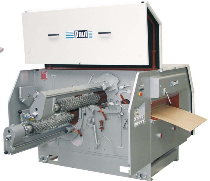
Saw shafts of the 'K34G-OUR' fitted with profiling tools
